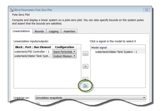
The block that originates the selected signal is highlighted in the Simulink model.
